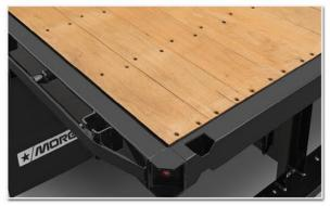
A standard, heavy-duty rub-rail helps to protect the flatbed frame and side rail pockets from minor impacts.
