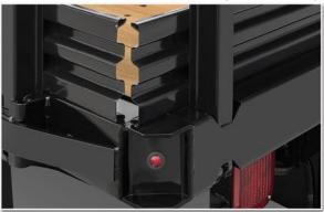
Heavy-duty Apitong wood flooring comes standard on all ProStake bodies, and offers natural shock absorption, weather and insect resistance.
