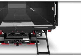
Stirrup steps at rear, roadside and curbside doors with anti-slip tape on floor for added traction
