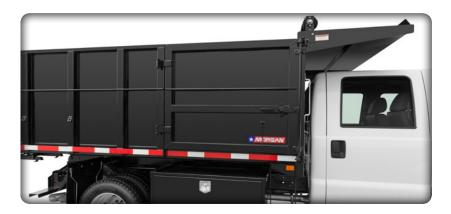
Side Door at curbside foremost location to swing towards rear with cam action lock hardware and door hold backs.
